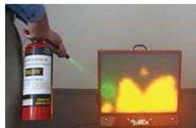
The system uses LED driven digital flames and lasers to simulate the discharge of actual extinguishers for a completely clean and safe training experience. Your trainees can enjoy effective training with the benefit of no increase to safety as no live fire is used.
